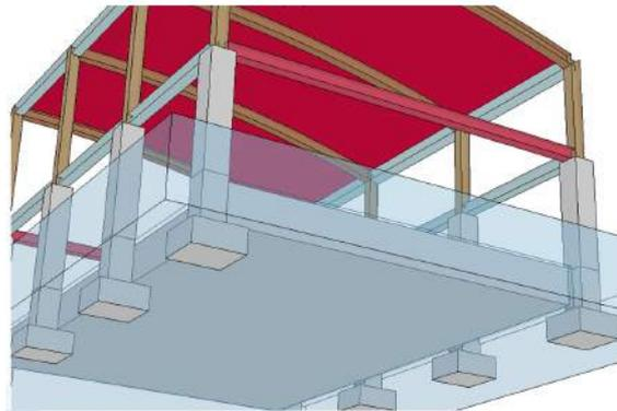
Concrete slab isolated from the 'rest of the world'
