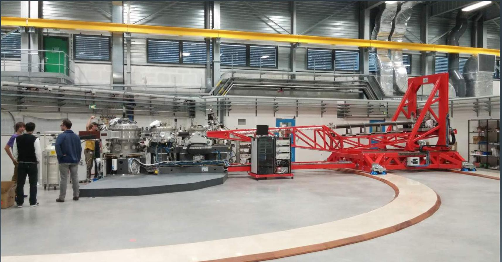
ID32 at the ESRF (Grenoble, France), 12 meters. A similar spectrometer, 15 meters in length, is currently in construction at NSLS-II.
