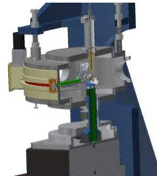
Sample and optics on granite blocks, decoupled from chamber
