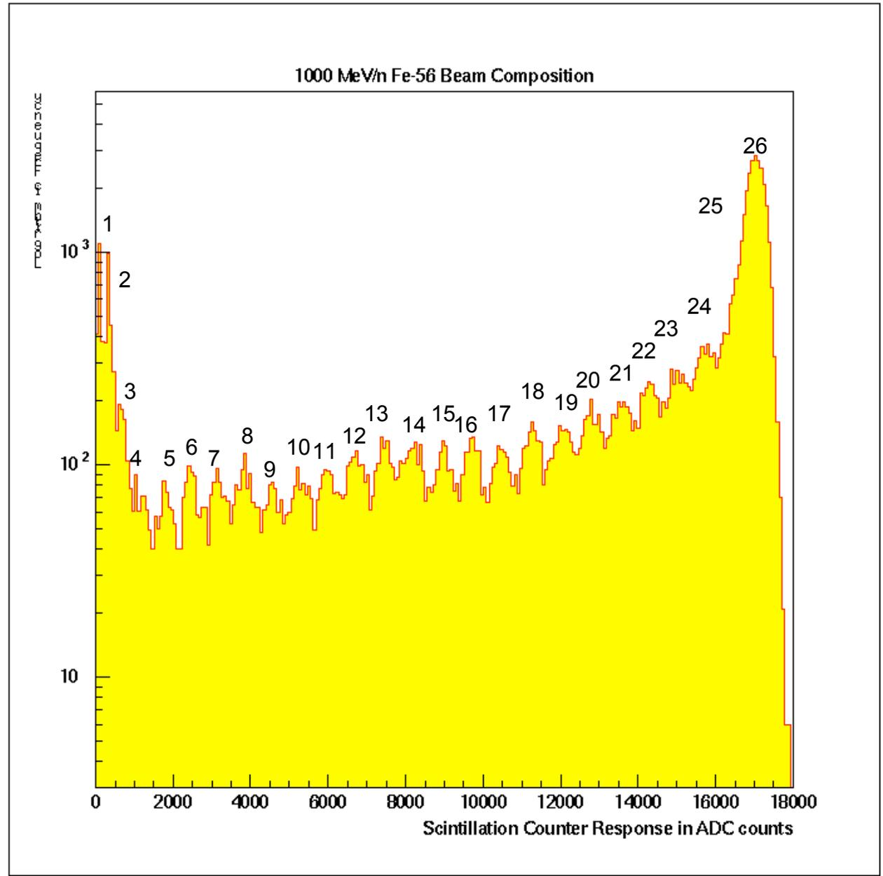
The LBL Silicon detectors have better energy resolution than scintillator, giving good separation between peaks of different Z.
