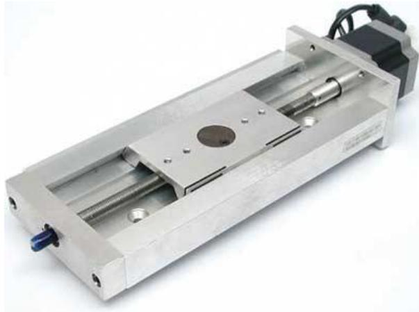
$$\text{MRES} = \left( \frac{\text{EGU's}}{1 \text{ leadscrew rev.}} \right) \times \left( \frac{1 \text{ motor rev.}}{\text{motor steps}} \right)$$
