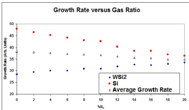
Figure 2. Growth rate of  $WSi_2$  and Si for concentrations of nitrogen from 0% to 20%.
