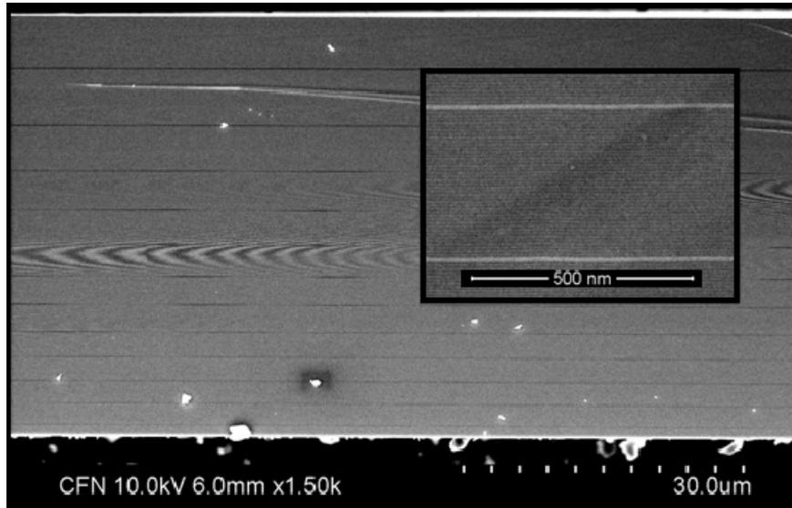
Figure 7. SEM image of a 43 $\mu$ m thick MLL with 12 marker layers inserted for layer placement metrology. The offset streak near the top is not a growth defect, but is due to polishing scratches.
