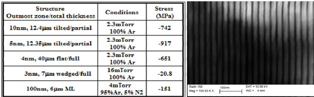
Figure 1. Accumulated film stress vs. structure, and evidence of waviness due to high pressure growth.
