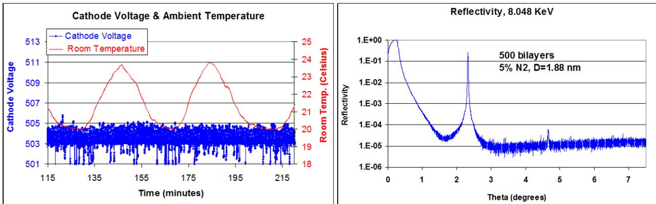
Figure 6. Applied cathode voltage is highly stable, even with room temperature swings of  $\sim 4^\circ$  C after installation of the gauge isolation enclosure, and the resulting x-ray reflectivity with clear evidence of high growth rate stability.
