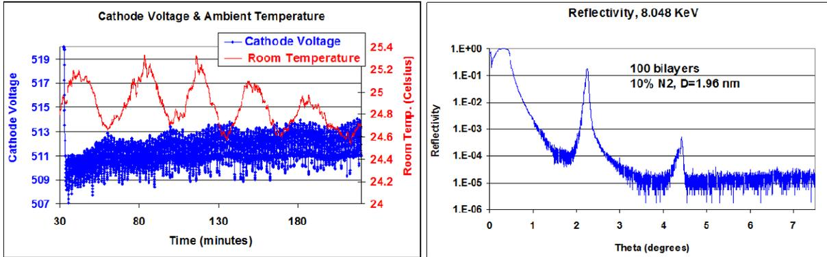
Figure 4. Applied cathode voltage fluctuations due to room temperature swings of  $\sim 0.5^\circ\text{C}$  before addition of the gauge isolation enclosure, and the resulting x-ray reflectivity with clear evidence of growth rate instability.
