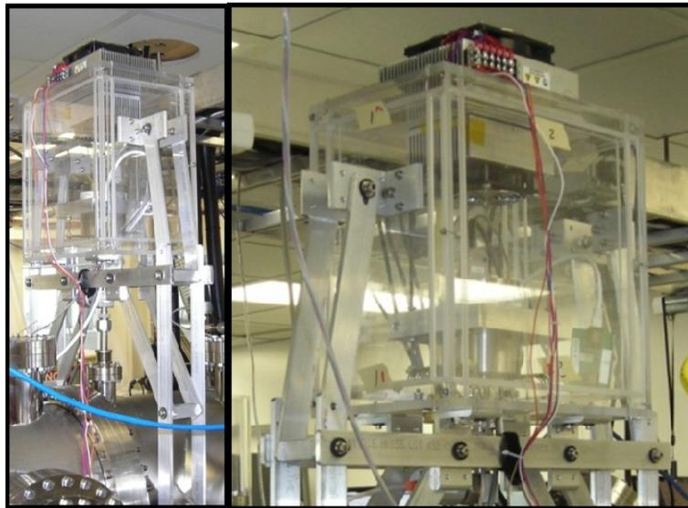
Figure 5. Double-walled acrylic temperature and vibration isolation enclosure for the capacitance manometer
