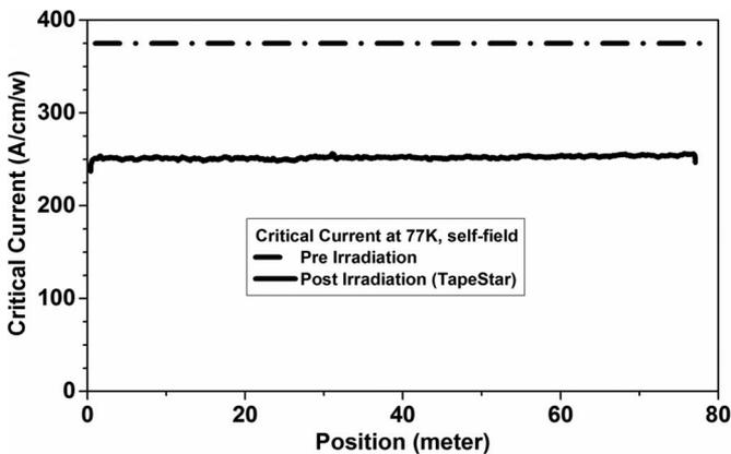
Fig. 6.  $I_c$  (77 K, self-field) as a function of length for a coil wire made from a 46-mm strip after irradiation to a dose of  $6 \times 10^{11}$  Au/cm<sup>2</sup>. The preirradiation value is estimated from pieces cut from the ends of the original 46-mm strip.
