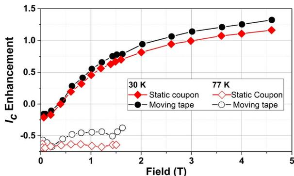
Fig. 2.  $I_c$  enhancement at 30 and 77 K (relative to an unirradiated control sample) of a stationary short sample and a moving 1-m tape after irradiation with 18-MeV Au to a dose of  $6 \times 10^{11}$  Au/cm<sup>2</sup>.
