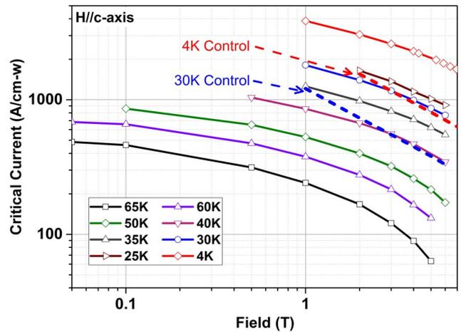
Fig. 7.  $I_c$  as a function of temperature and field (H//c) for a Au irradiated wire.  $I_c$  values for unirradiated control samples at 4 and 30 K (dash lines) are included for comparison.
