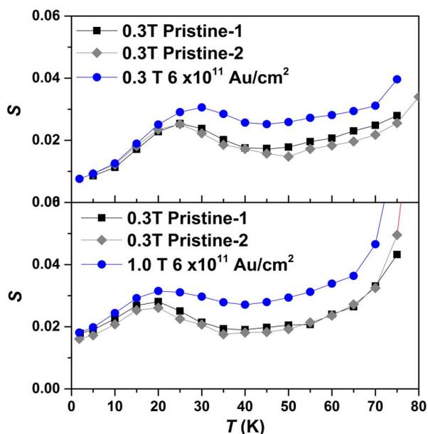
Fig. 3. Flux creep rate as a function of temperature for an Au irradiated sample at 0.3 T (upper figure) and 1.0 T (lower figure).  $S(T)$  for unirradiated controls are included for comparison.
