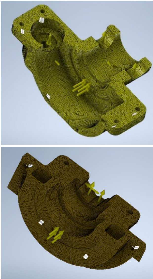
Figure 5: Finite Element mesh with applied force vectors for one half of (a) the housing and (b) housing plate that retains the worm and ring gear mechanism.
