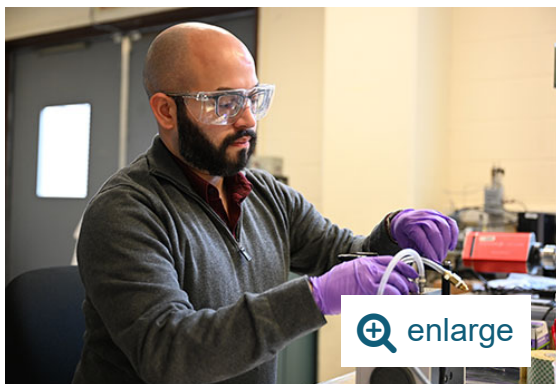
Juan Jimenez assembling the high-pressure gas-solid-liquid infrared spectroscopy cell in the Chemistry Division laboratory. (Kevin Coughlin/Brookhaven National Laboratory)
