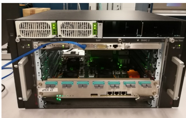
Figure 8. Fully assembled gFEX prototype v3 board in the ATCA chassis with IPMC card; the board can be remote power cycling through the ATCA shelf manager.
