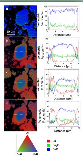
Left column: Chemical phase mappings of a CuO anode during cycling. Right: Line profile showing the corresponding chemical changes of an anode particle.
