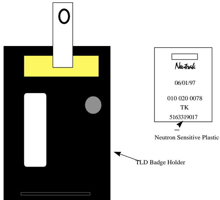
The TLD **monitors** your exposure to beta, gamma, and neutron radiation. It offers **no protection** from radiation.
