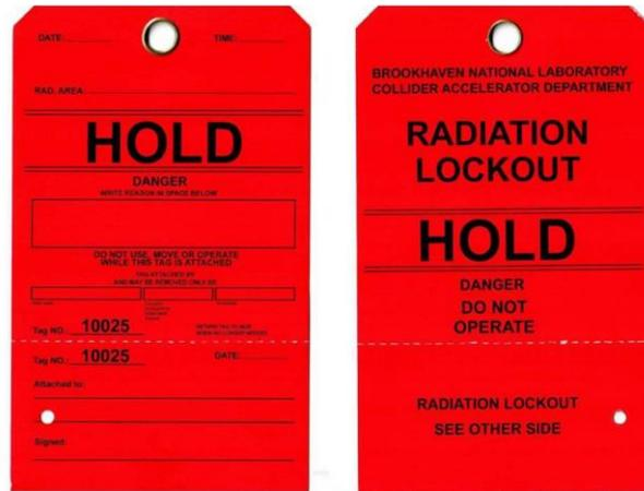
CA D also uses Radiation Safety Lockout/Tagout at the Medical Isotope Research and Production facilities (BLIP, RRPL, MIRP Cyclotron) and the ATF. RS-LOTO tags are used to inform and warn personnel at MIRP of equipment that is isolated or configured to provide radiation protection to personnel and to satisfy Accelerator Safety Envelope (ASE) requirements. RS-LOTO is to prevent unauthorized changes to this equipment and has specific application requirements at MIRP facilities and the ATF.
