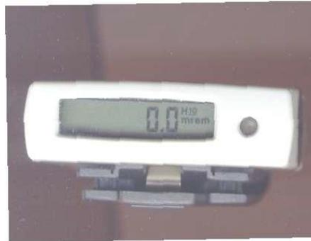
The purpose of the self-reading dosimeter is to allow personnel to monitor their own exposure and compare it to the daily C-AD administrative control level (ACL) of 100 mrem. Self-reading dosimeters have  $\pm 20\%$  accuracy for gamma. They only respond to gamma. They are not calibrated to measure neutrons.
