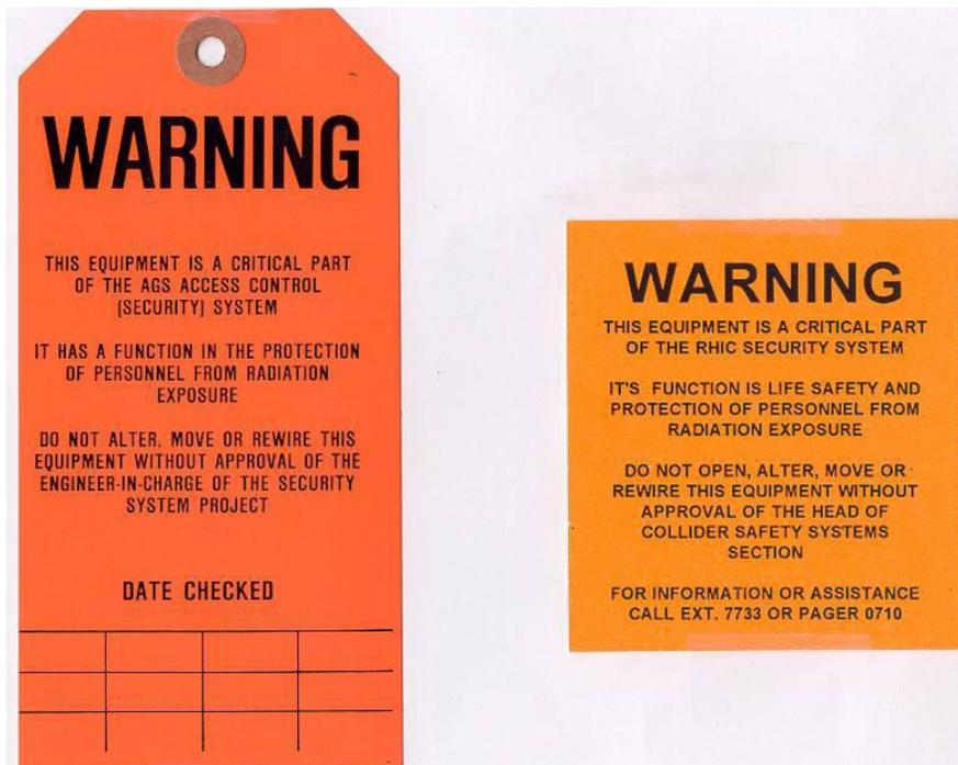
In addition to an orange warning tag, equipment specialists document allowable work, such as routine maintenance, that may be performed on ACS equipment. Equipment specialists provide this information for each piece of equipment they connect to ACS. The Access Controls Group makes these informational documents available to all personnel who work on the equipment. C-
