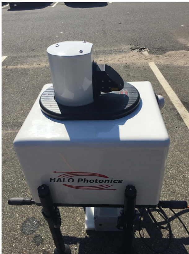
Figure 14: BNL long range Doppler LIDAR
