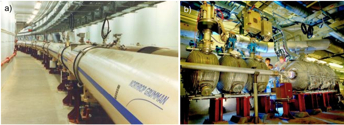
Figure 2.2.: a) The two RHIC rings, consisting of hundreds of magnets, inside the tunnel. b) One of the two radio frequency cavities [30].
