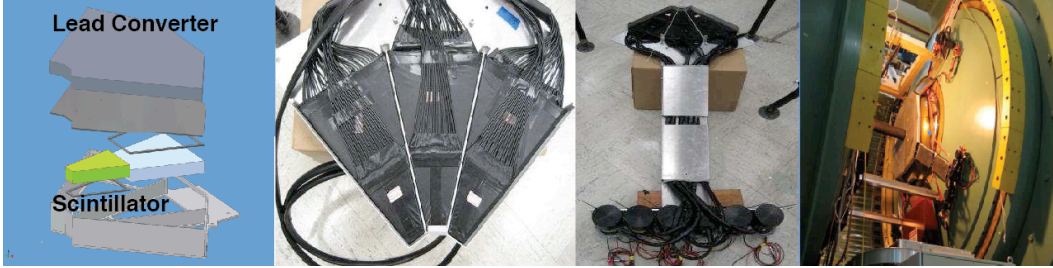
Figure 2.8: RXP construction. PbSc paddle (left), a partial ring of paddles (left-center), paddles with PMTs attached (right-center), and the RXP as installed in PHENIX (right). [74]
