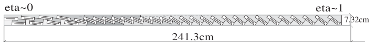
Figure 2.6: Layout of MRPCs in a single TOF tray
