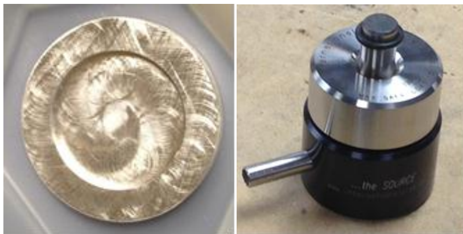
Figure 2.1.2. (left) Aluminum backing used for target irradiations (right) 13 mm pellet die used to prepare pressed targets
