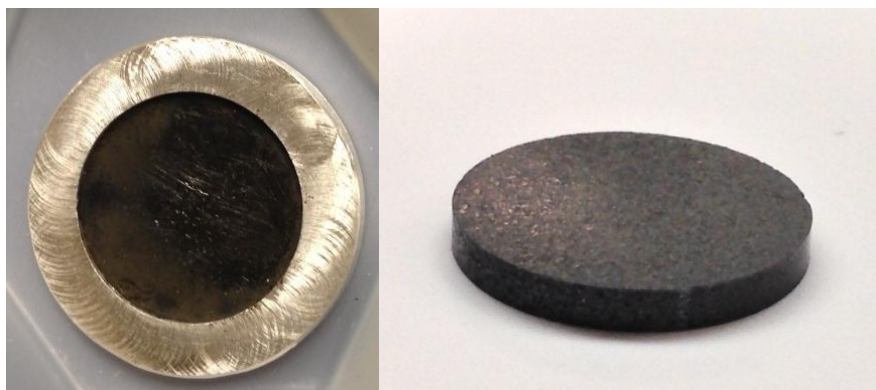
Figure 2.1.5. (a) OsS 2 pressed directly into backing (b) pressed pellet of OsS 2 which is transferred to target backing
