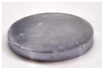
Figure 4.2.1. Thick MoS 2 pellet pressed using the pellet die
