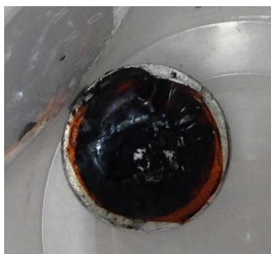
Figure B.3.2. \text{OsS}_2 target with burnt foil and wet target material
