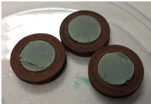
Figure 2.2.1. Pressed ^{nat}\text{WO}_3 disc in tungsten alloy backing (post-sintering)
