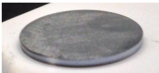
Figure 2.2.3. Pressed disc of tungsten disulfide
