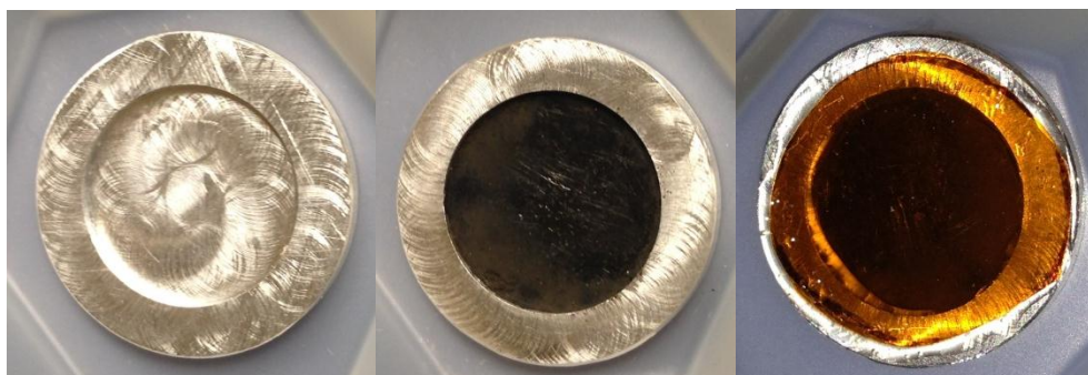
Figure B.3.1. (Left) empty aluminum backing (Middle) \text{OsS}_2 pressed into aluminum backing (Right) Target coated with Kapton foil epoxyed to the surface
