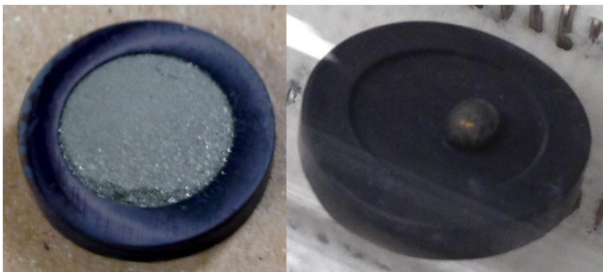
Figure 3.1.3. (left) sintered Ge pellet (right) annealed Ge mass
