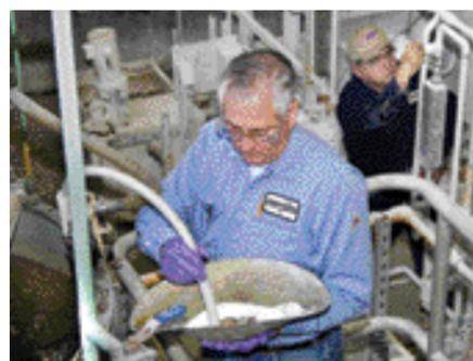
**STEP 5.** Polymer is added to aid in flocculation (see step 6). Richard Lutz (front) adds polymer into a rapid-mix tank, as Phil Pizzo adjust the flow rate. — D2810306
