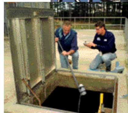
**STEP 10.** At the clear well, where up to 250,000 gallons of "finished" water is stored before its final chlorination and distribution, Richard Lutz and Jack Kulesa take samples. — CN10-146-00
