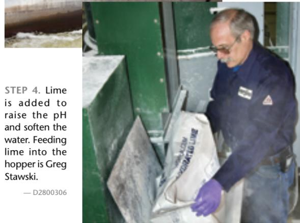
**STEP 4.** Lime is added to raise the pH and soften the water. Feeding lime into the hopper is Greg Stawski. — D2800306
