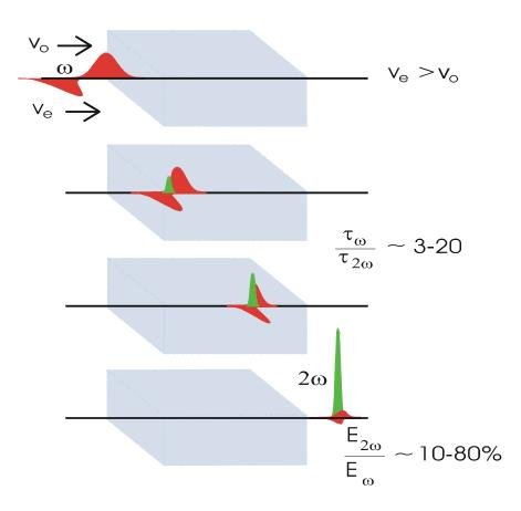
SNLO code simulations of 1064 to 532 nm conversion in 10 cm crystal with group velocity mismatch.
