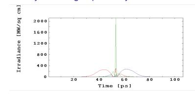
•Measured compression from 1 micron to 532 nm with pulse duration decrease of 3-4x in a 10 cm KD\*P doubler.
