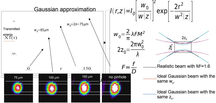
•Laser focus transmitted through pinholes of 75-150  $\mu$ m dia imaged on IR camera. Gaussian approximation with w<sub>0</sub>=65  $\mu$ m is the best fit to the observed transmission through pinholes. For ideal diffraction-limited beam, such focus corresponds to F<sub>#</sub>=10 and double Rayleigh distance 2.5 mm. Instead, we measure 2z<sub>0</sub>=0.8 mm and F<sub>#</sub>=4. This means that the beam has M<sup>2</sup>=1.6.
