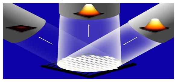
A micromirror array as used in commercial projectors is robust enough to serve as an active beam shaper for a laser beam.
