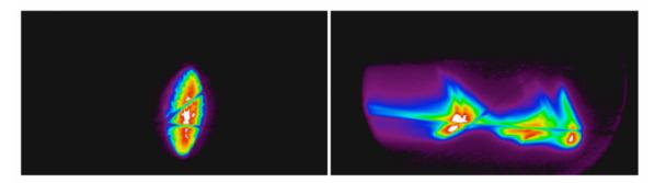
Min. energy spread and no compression - 9 deg fwd of crest (left); Max. compression -19 deg fwd of crest (right).
