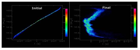
Parmela-Elegant simulation longitudinal phase space of beam, with compression from 50A to 1.5 kA.
