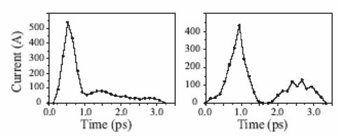
Longitudinal Distribution for compressed (left), and over-compressed (right) cases.
