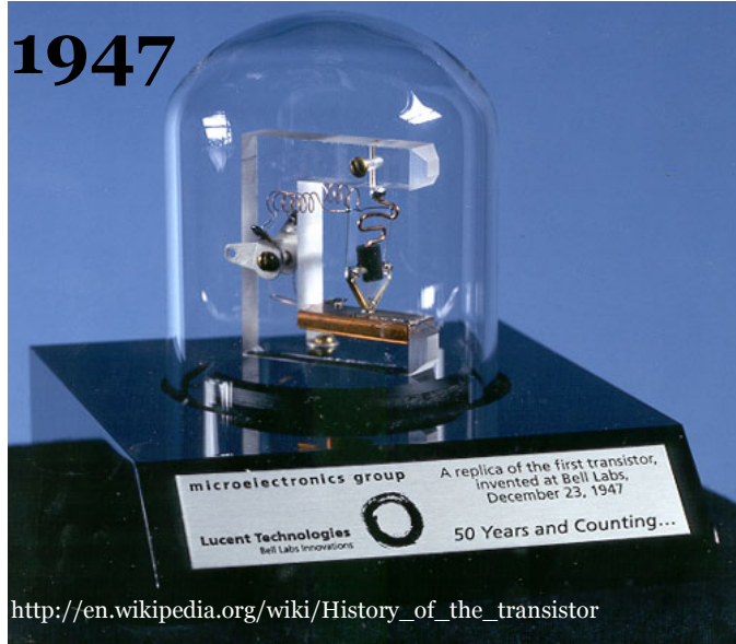
A replica of the first transistor
