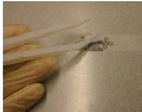
Gentle Rubbing with plastic Tweezers
