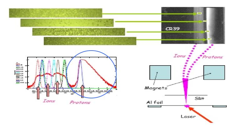
Proton and ion energies were diagnosed with a compact magnetic spectrometer followed by a CR39 plate. A density plot obtained with a scanner is overlaid with artificial peaks that illustrate the expected position and spread due to a finite spectrometer slit for the 1-MeV protons and any possible Al+n and C+n ions accelerated in the same field.
