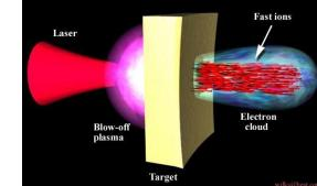
Physics of ion (proton) acceleration by a laser in a foil target: TNSA
