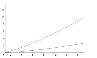
Proton energy (MeV) vs laser power (TW). Red is for 10 μm, blue is for 1 μm
