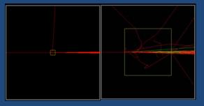
100 $\mu$ m thick fiber (left) and 1mm thick fiber (right). Red lines are e<sup>-</sup> trajectories.
