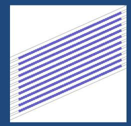
Fiber layout with ~10µm shifts between layers
