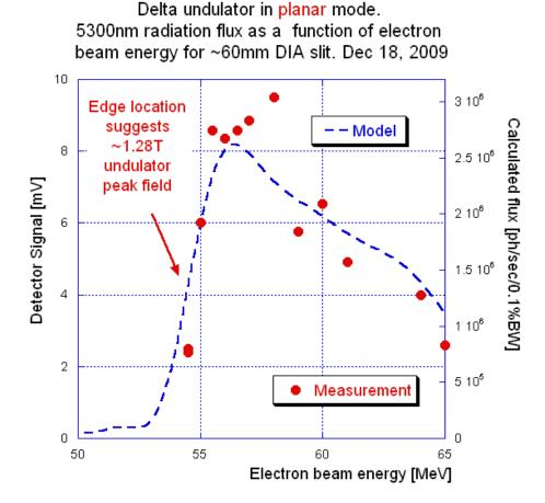
5300nm wavelength radiation intensity on axis as function of the electron beam energy.
