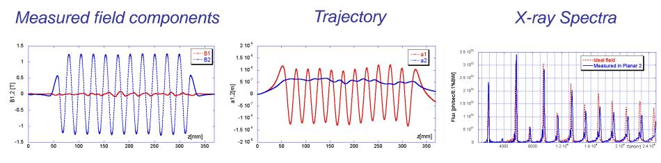
Planar mode, - 45deg linear polarization (phase between vertical and horizontal pairs 180deg)
