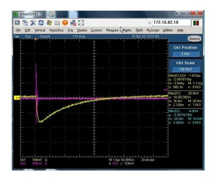
Infrared radiation detected by InSb sensor
