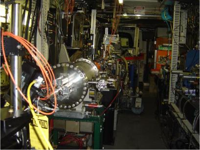
Delta undulator installed in BL2 at ATF.
