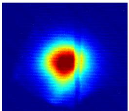
Electron beam downstream of undulator
