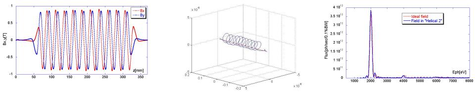
Helical mode, right circular polarization (phase between vertical and horizontal pairs -90<sup>0</sup>)
