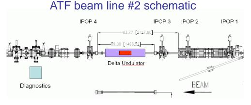
ATF beam parameters: Energy in range from 52MeV to 72MeV Normalized emittance 1e-6 m\*rad Bunch charge ~ 500pC Repetition rate ~ 1.3 pulse/sec
