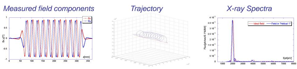
Helical mode, left circular polarization (phase between vertical and horizontal pairs 90°)
